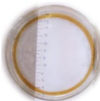
Fig. 7- Oil displacement test for B. velezensis UTB96 supernatant grown in modified medium
