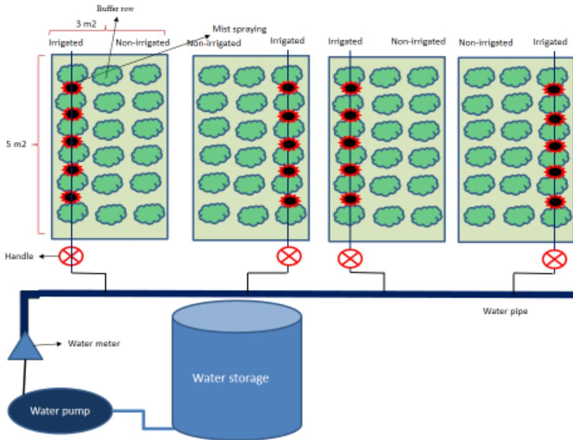
Fig. 1. Schematic of the irrigation system
